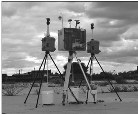
Monitors measure dust and hexavalent chromium concentrations.
